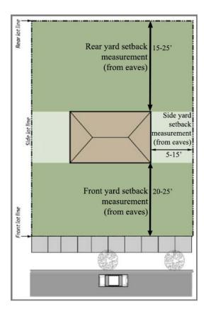
The diagram above will reflect how you will be required to measure your setback. Do not measure from the footprint, but instead from the furthest edge of the structure. If there are roof eaves, measure your setback starting at the edge of the roof eaves. If there is a built in porch or balcony, the same rule applies to those extensions of the structure.
