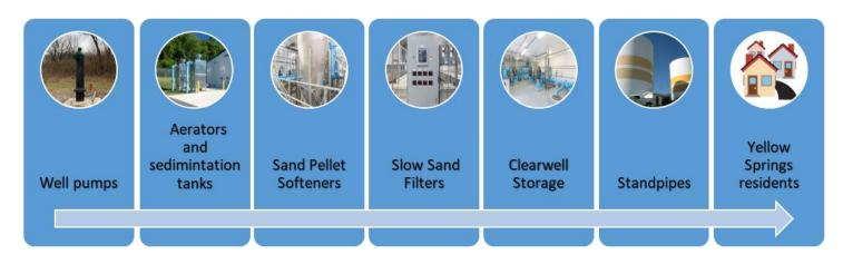
Yellow Springs water is groundwater that is produced from 5 wells located along the Little Miami River near Jacoby Road. The wells vary in depth from 60′ to 130′. The raw water is pumped to the Water Treatment Plant, where it is aerated, softened, filtered, and disinfected prior to it being pumped to the water customers of the Village of Yellow Springs.
